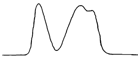
Figure 6.—Gas chromatography of methyl, ethyl and isopropyl benzoates 190°C.
