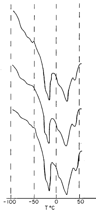
Figure 3. Reproducibility test for the apparatus. Successive plots from the same sample.
