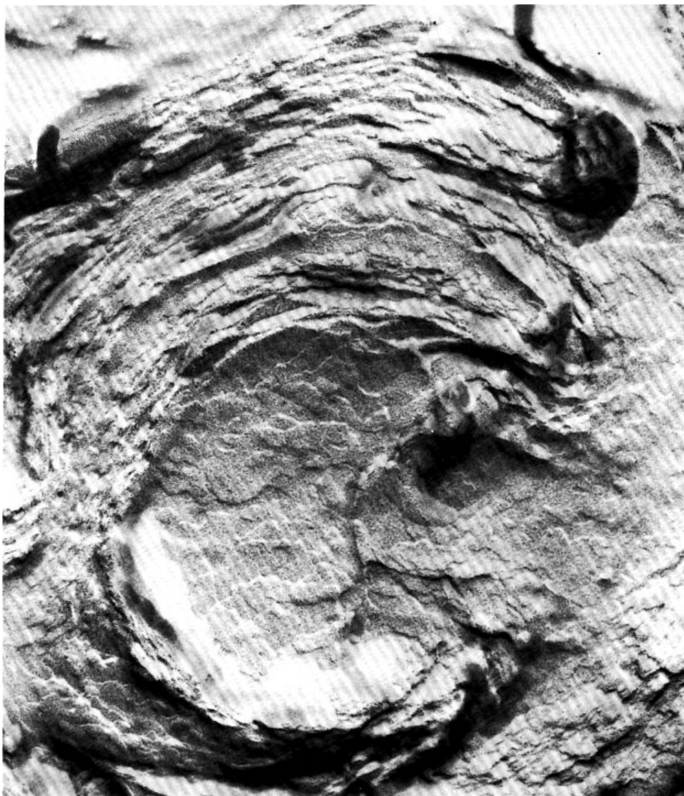
Figure 6. The liquid crystalline layers in an emulsion may be directly observed in an electron microscope photograph of the carbon replica from freeze-etched samples.
