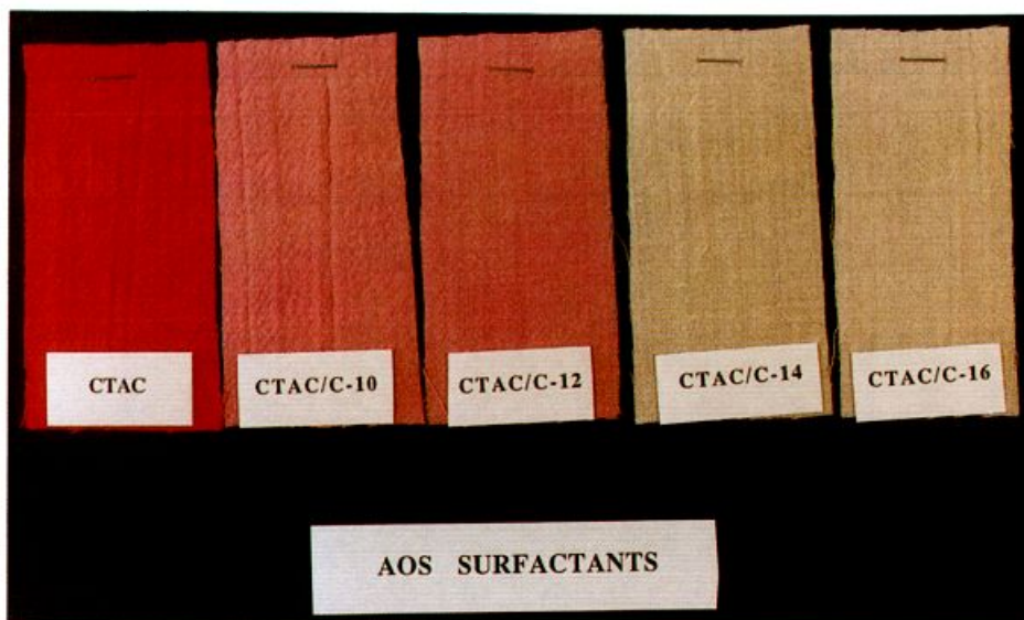
Figure 4. Wool swatches stained with Red-80 dye after treatment with CTAC and washing with AOS detergents.
