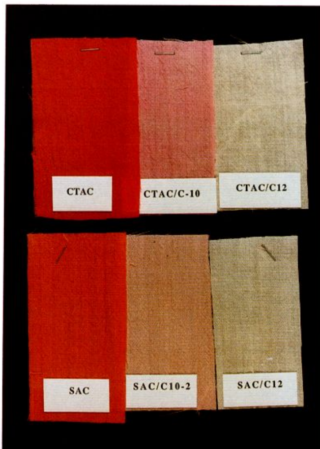
Figure 2. Wool swatches stained with Red-80 dye after treatment with either CTAC or SAC and washing with C10[SDES] or C12[ALS] detergents.
