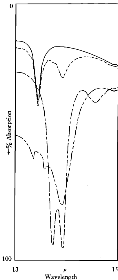
Figure 3.—Absorption spectrum of Utah wax: — iso-octane, solvent; --- Utah Wax in iso-octane; ——— Utah Wax, solid, room temp.; - - - - Utah Wax, molten, 120°.
