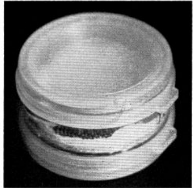
Figure 2.—Desiccator fabricated from a glass cylinder, covered with polyethylene snap cap.
