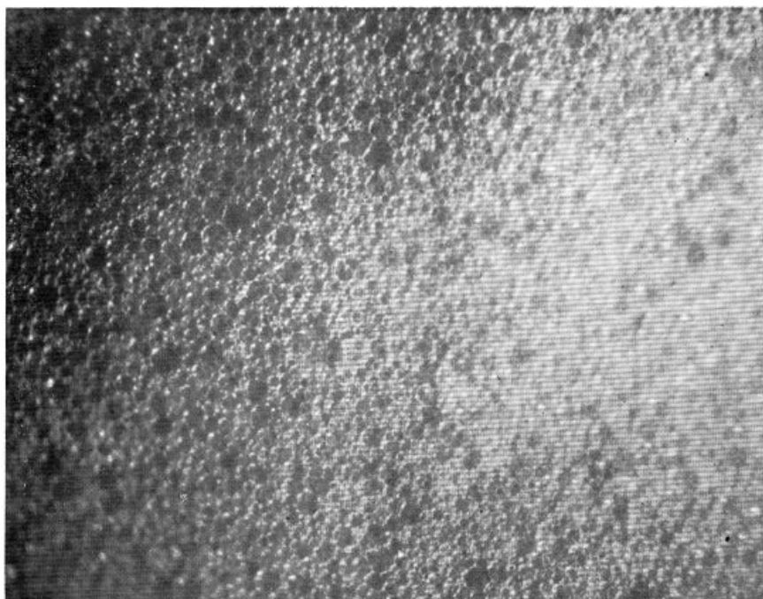
Figure 4. Photomicrograph of a sodium lauryl sulfate/lauryl alcohol foam with Freon-12/Freon-114 (40/60) propellant
