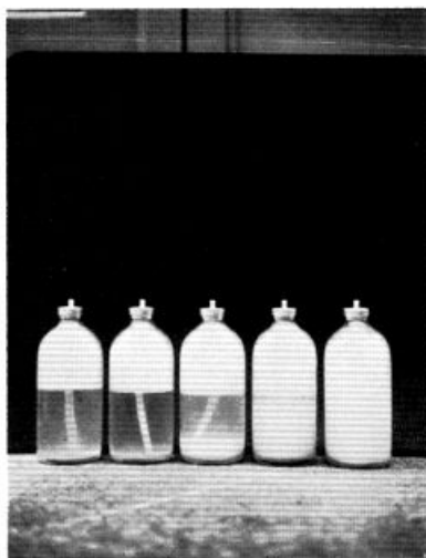
Figure 3. Comparative emulsion stabilities of sodium lauryl sulfate systems with increasing concentrations of lauryl alcohol (from left to right). The picture was taken four hours after the samples were shaken
