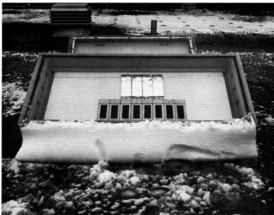
Figure 2. Two shielded and four exposed sample hair groups in sunlight exposure box
