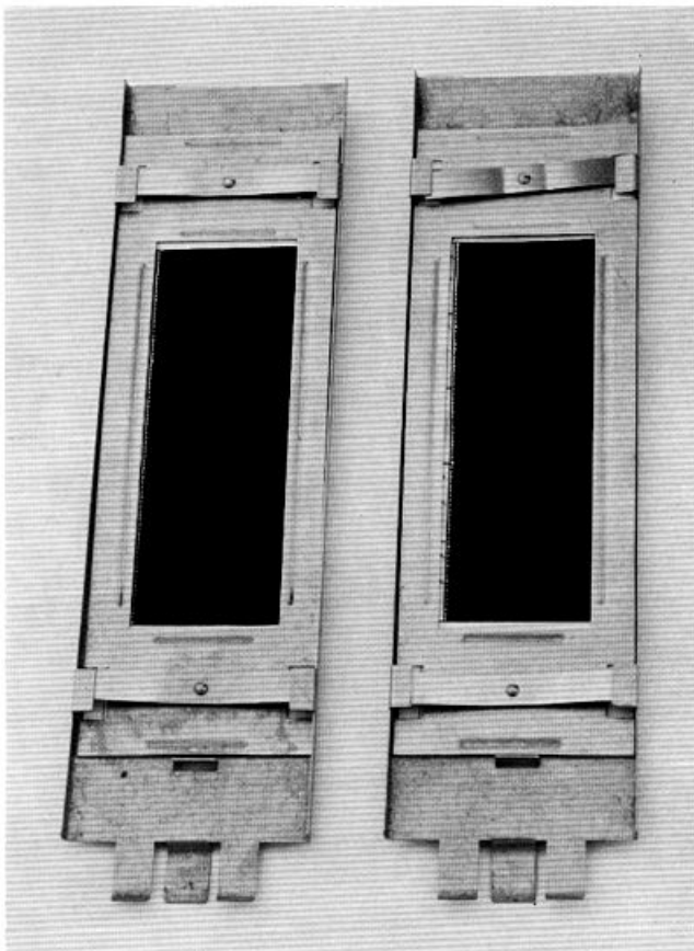
Figure 3. Sample hair group mounted in Atlas SL-LSR specimen holder
