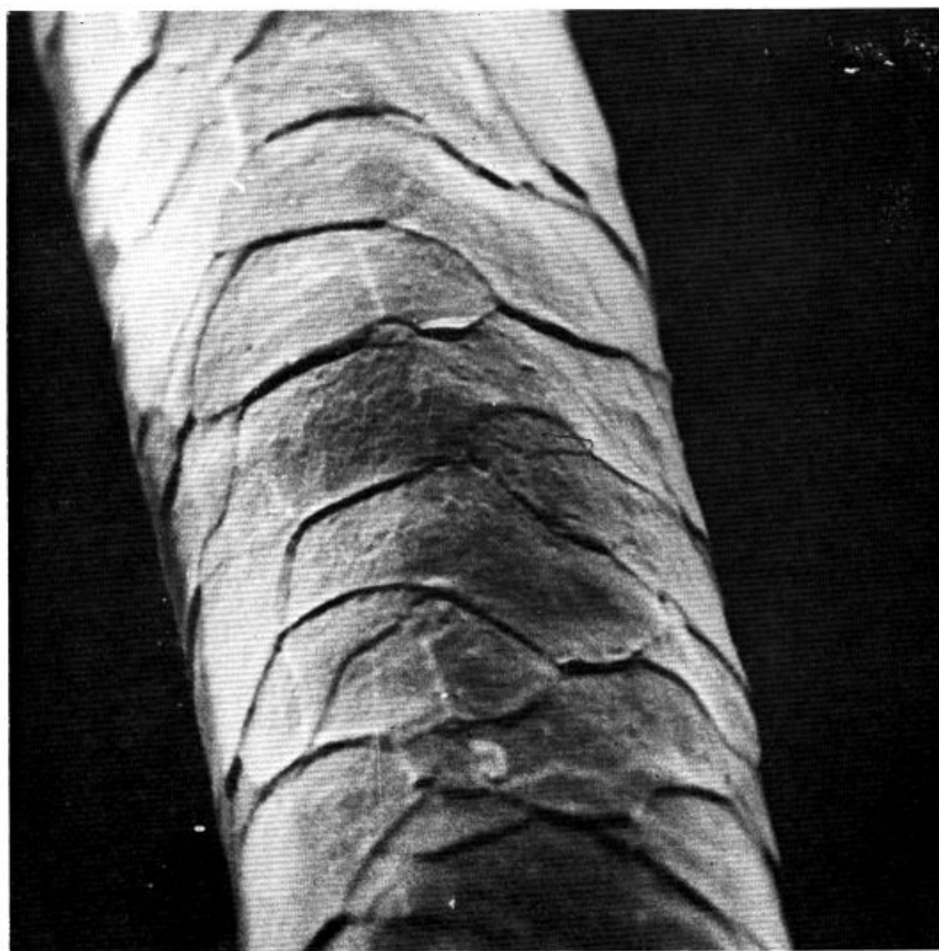
Figure 6. Scanning electron micrograph of intact mohair. Magnification, 2750
