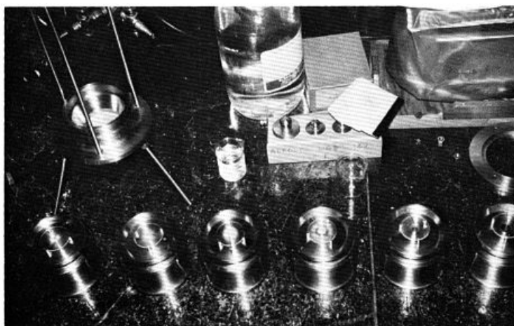
Figure 3. Cascade Impactor disassembled showing glass slides
