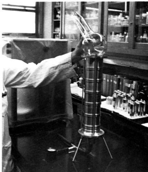
Figure 1. Assembled Cascade Impactor fitted with sampling chamber
