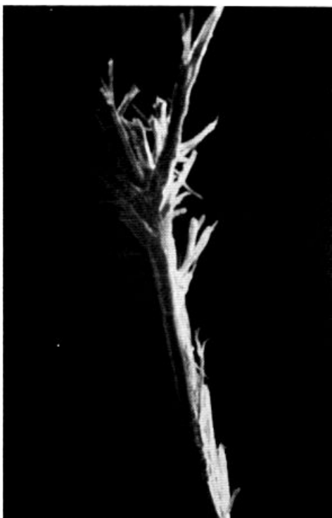
Figure 6. Damage category—flyaway fibers
