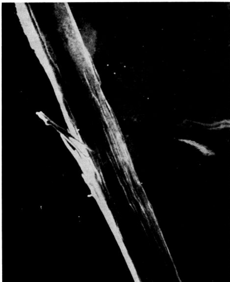
Figure 11. Micrograph of same area as in Fig. 10 showing repair of shaft damage with one application of conditioner
