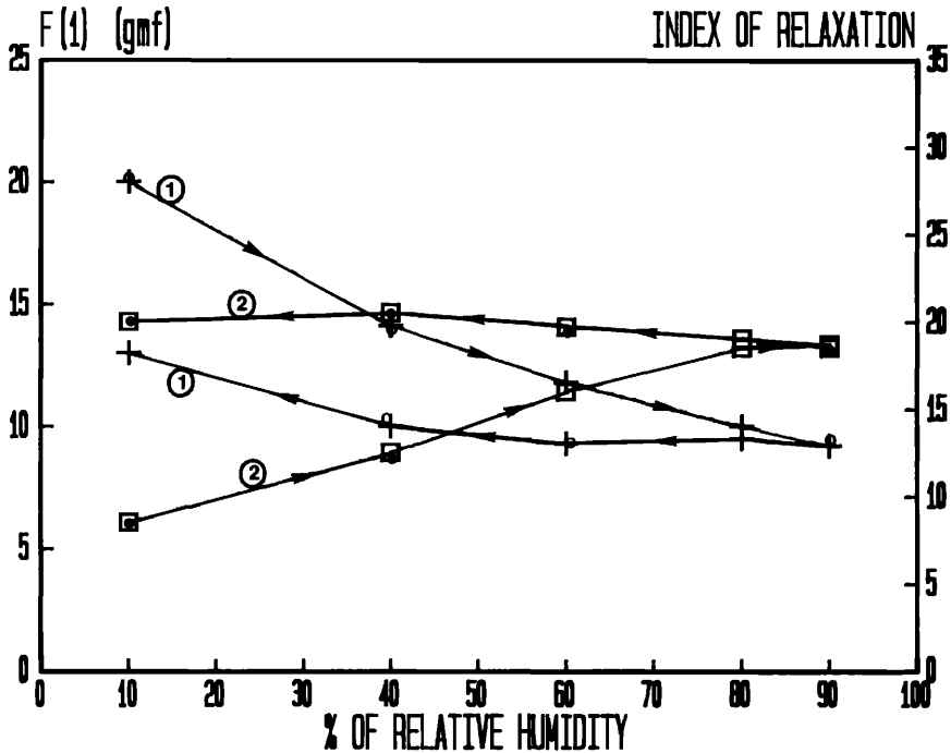
Figure 14. Hysteresis curves of fibers treated as follows: F(1) - (1 +), and IR - (2 □), after 10-minute treatment in 100% glycerine; and F(1) - (1 ○), and IR (2 ●), after 10-minute treatment in 100% propylene glycol.
