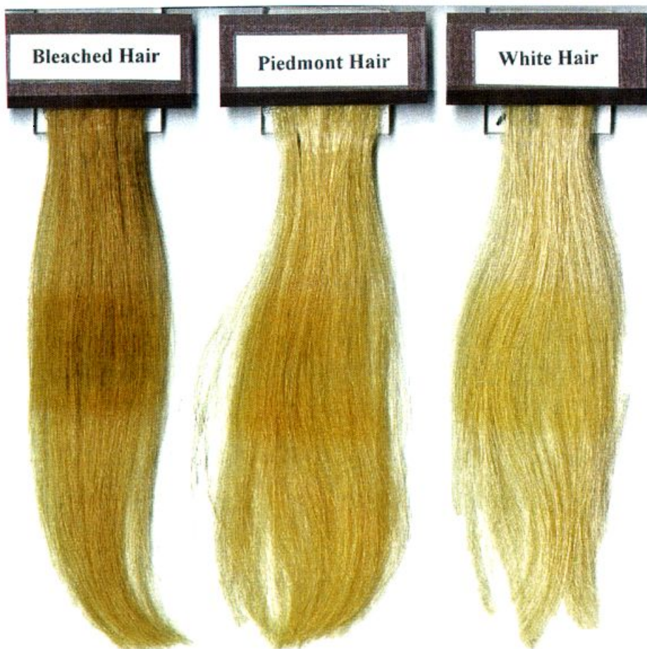
Figure 9. Bleached, Piedmont, and white (unpigmented) hair after 30 min (5-min intervals) of thermal treatment at 164°C.
