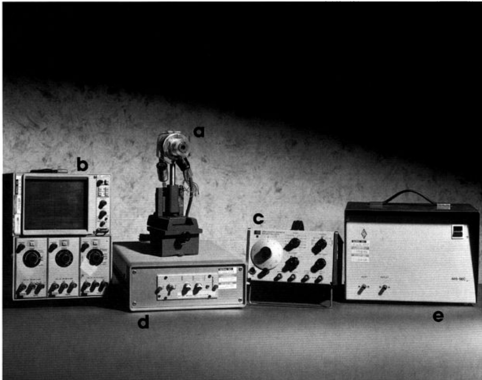
Figure 1. Equipment used in a GBE workstation: a, GBE probe; b, storage oscilloscope; c, function generator; d, signal conditioner; e, air compressor.
