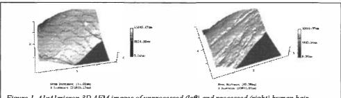
Figure 1. 41x41micron 3D AFM images of unprocessed (left) and processed (right) human hair structure.
