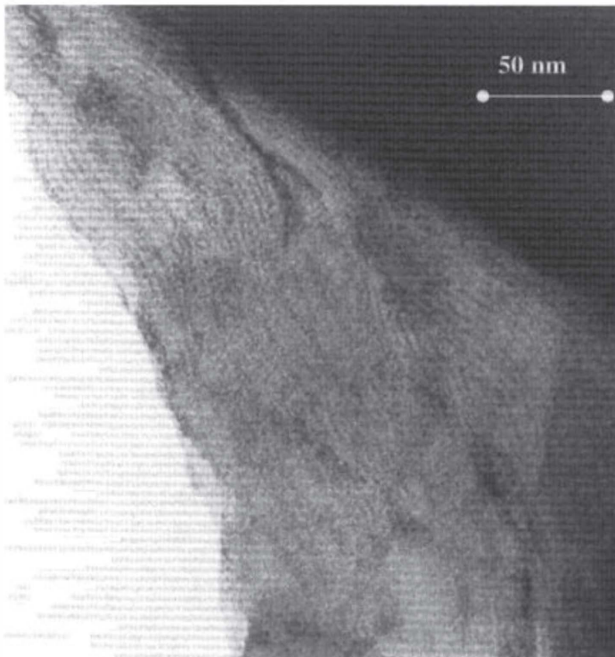
Figure 4. TEM micrograph of microfibrils in medulla parallel oriented to the section.
