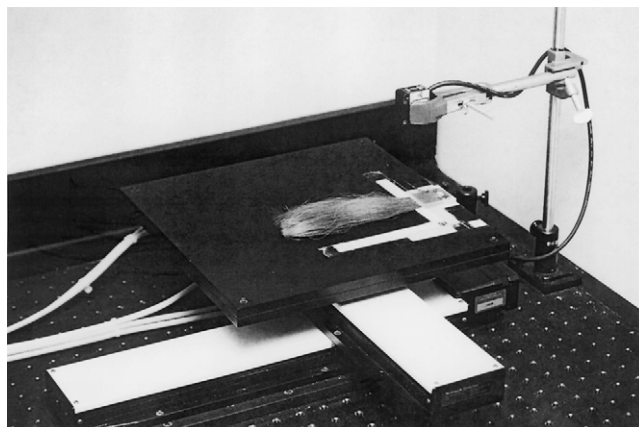
Figure 1. Photograph of the three-dimensional laser stereometer.
