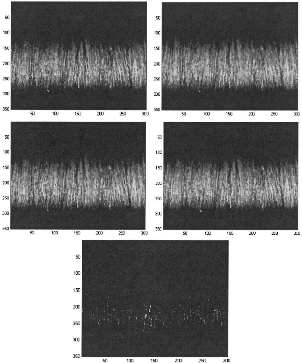
**Figure 3.** Determination of sparkle. The upper four photographs show the absolute intensities recorded for the same hair tress under four slightly different incident angles. The lower picture shows the standard deviations of the means of all individual pixels from the upper four pictures.
