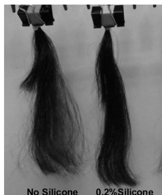
Figure 11. Tress photograph after 3 iron cycles at 154°C, 1 wash, and storage for 30 min at 90% RH. {Note: Test data. Actual results may vary.}
