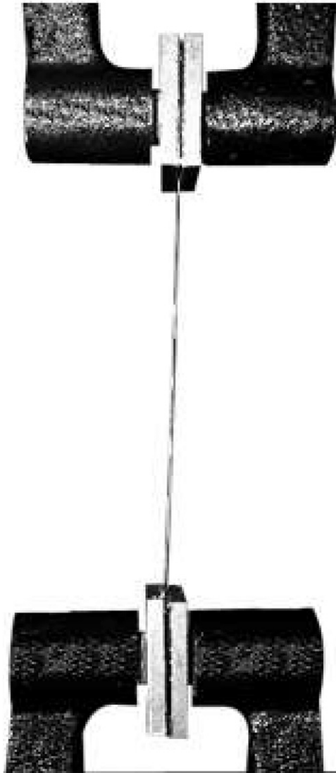
Figure 17. Photograph of pneumatic clamps of an Instron tensile tester containing a mounted hair fiber.
