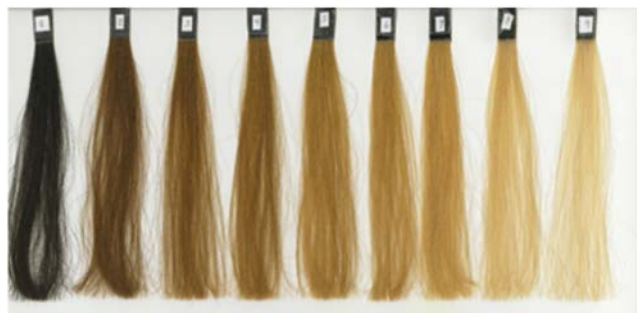
Figure 2. Photograph of (1) European dark brown hair, and European dark brown hair bleached for (2) 15 min, (3) 30 min, (4) 45 min, (5) 60 min, (6) 90 min, (7) 120 min, (8) 180 min, and (9) 240 min. For the series of tresses, a plot of \Delta E as a function of the kynurenine fluorescence intensity ( I_{440}/I_{339} ) resulted in a linear relationship of increasing slope with very good correlation ( R^2 = 0.91 ).
