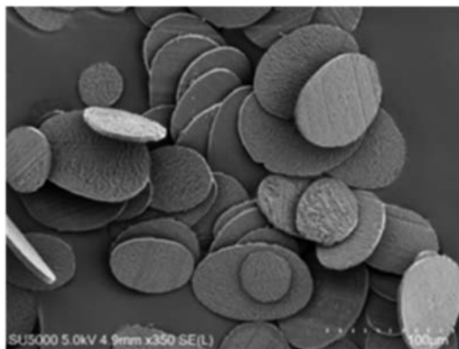
Figure 1. FESEM image of European dark brown hair fiber cross-sections (courtesy of W.T. Thompson, Ashland Specialty Ingredients, G.P.).
