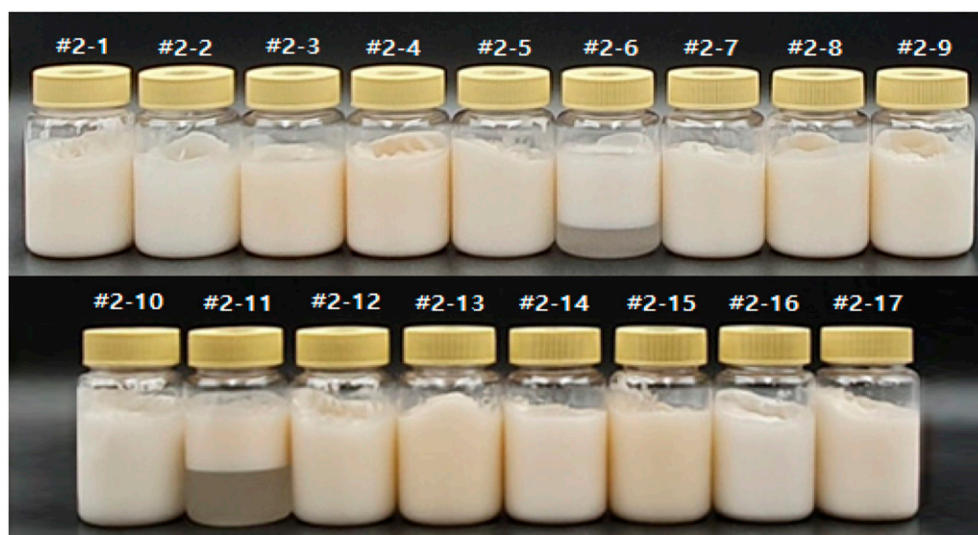
Figure 5. After 3 weeks' stability at low temperature (4°C) (PLO gel #2).
